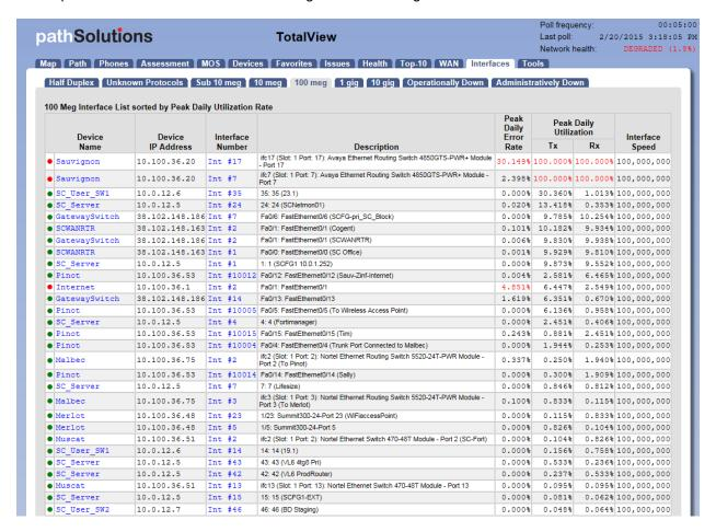
The highest utilized of these interfaces should be considered for upgrading to Gigabit Ethernet.
