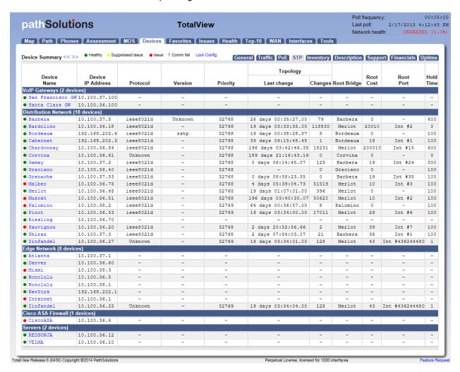
Determine when your last STP root bridge election occurred and which device is acting as the root bridge. Also know which interfaces are active as well as listening so you don't cause a reconfiguration by disconnecting the wrong interface.
