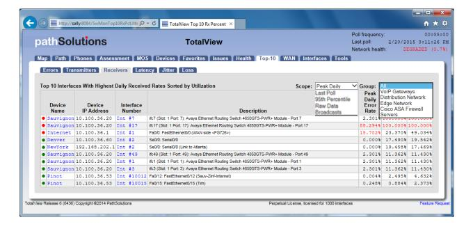
**Note:** If you have an interface that is receiving a high level of broadcasts, investigate the device that is connected to it to determine why it is transmitting a lot of broadcasts.
