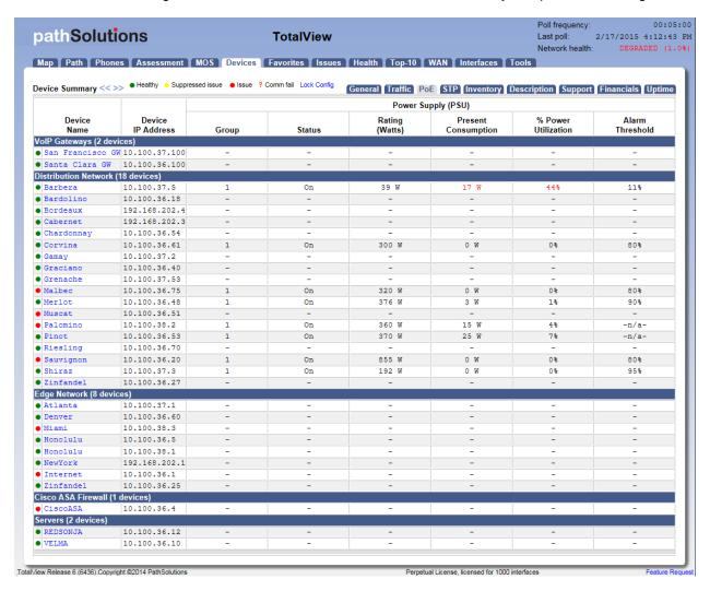
This allows you to quickly determine if there are any high-power drawing devices that are connected to the switch or if there are any power faults.
