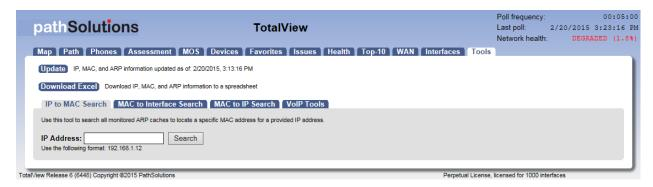
Before using any of the tools, you should click on the "Update" button to collect the Bridge table and ARP cache information from your network.
