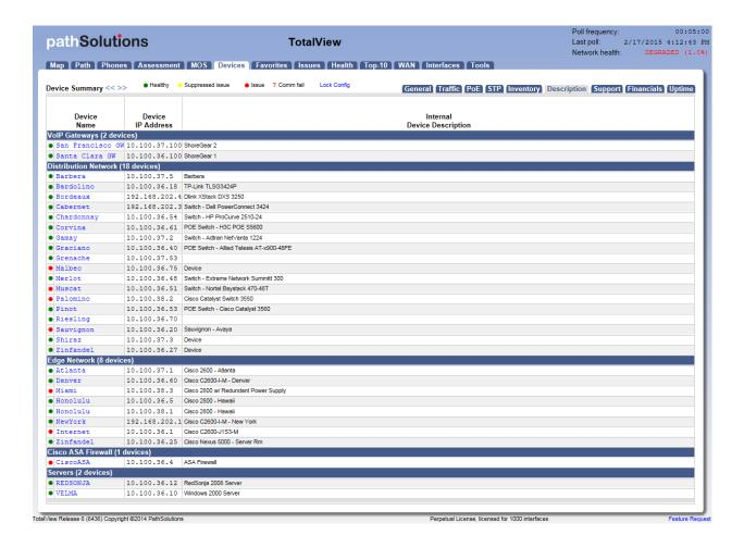
If a device goes offline and all that you see is a red?, you will no longer see any SNMP device name or information. Manually typing in a Device Description using the Config Tool will allow you to see a description on what device went offline.
