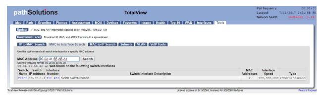
Notice that the MAC address was discovered on more than one interface. The "MAC Addresses" column will help you to determine how many MAC addresses exist on an interface. This is useful for determining if an interface is a switch to a switch trunk. If so, then more than one MAC address would exist on the link. If it is the interface where the device is physically connected to then there will only be one MAC address connected.
