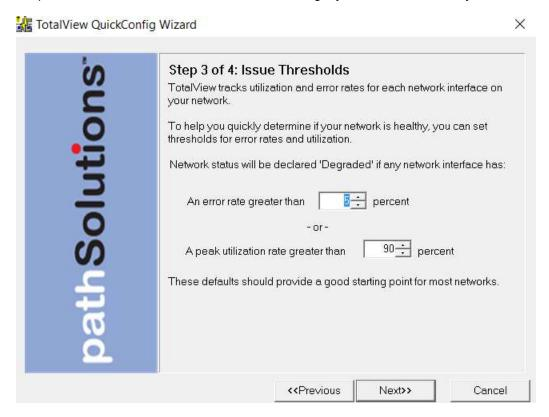
If an interface has an error rate higher than 5%, network status will be changed to 'Degraded'.
