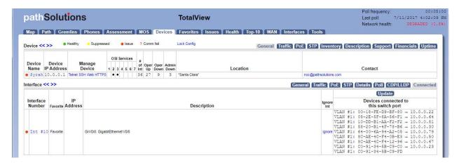
If determining the source and destination of the traffic is not enough to narrow down the cause, the next step would be to connect a network analyzer to that interface to try to determine the purpose of the traffic.
