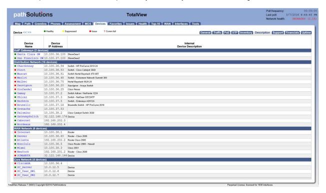
If a device goes offline and all that you see is a red?, you will no longer see any SNMP device name or information. Manually typing in a Device Description using the Config Tool will allow you to see a description on what device went offline.
