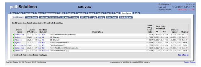
These interfaces should be converted to run in full-duplex mode to eliminate packet loss due to collisions.
