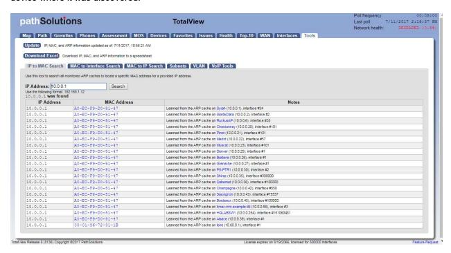
The MAC address will be displayed along with the device and interface where the MAC address was found in the device's ARP cache.
