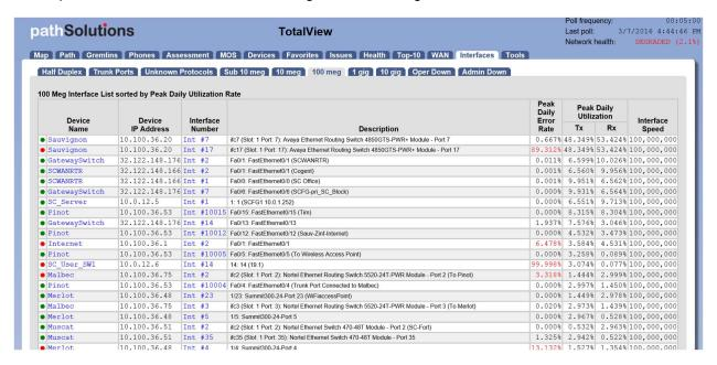
The highest utilized of these interfaces should be considered for upgrading to Gigabit Ethernet.
